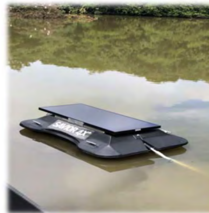
HyOx Floating Oxygenator GPS Solar Powered Drone
